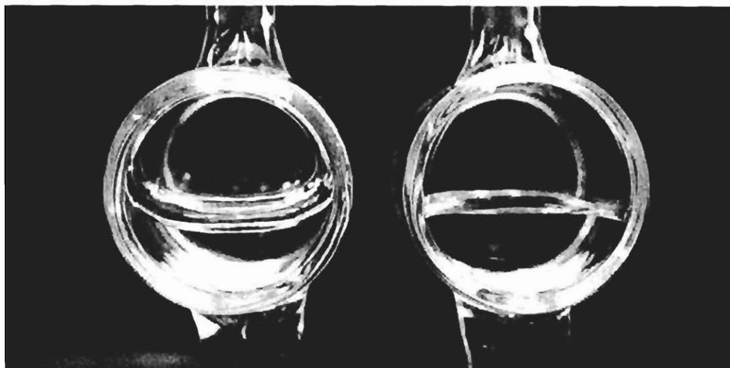
Figure 5-12: DI water inside an uncoated (left) and a coated (right) pump bulb. Clearly the water does not stick to the coated surface and the shape of the water surface is dramatically affected.
