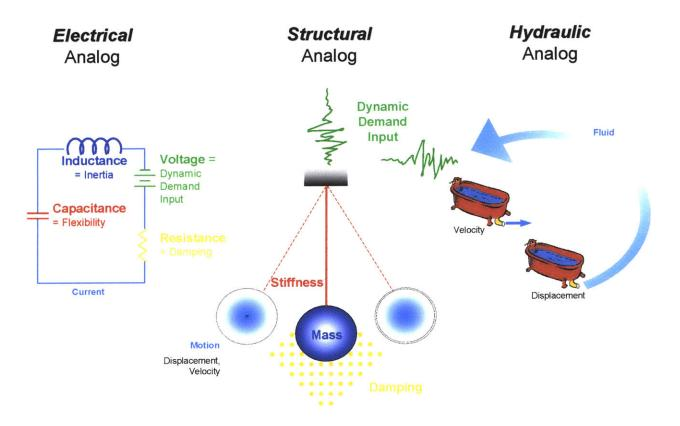
Figure B1: Equivalence of Hydro-Electro-Mechanical Systems
