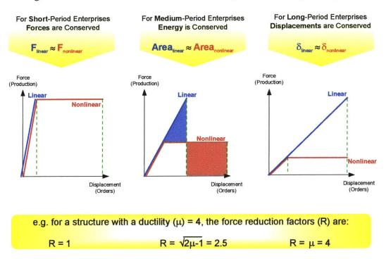
Figure 2.42: Newmark's Method for Constructing Nonlinear Response Spectra
