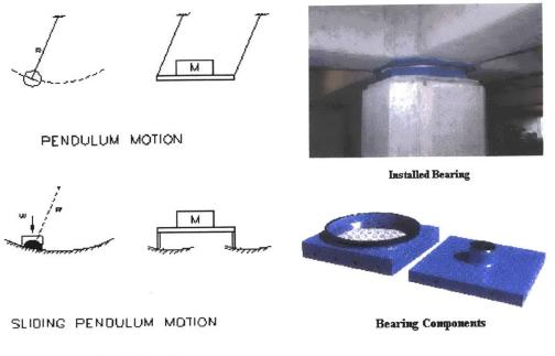
Figure 9.20: Friction Pendulum Base Isolation System (source: EPS Inc.)
