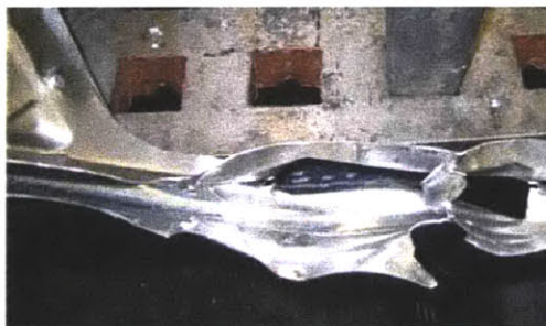
Figure 8. Destructive Weld Test
