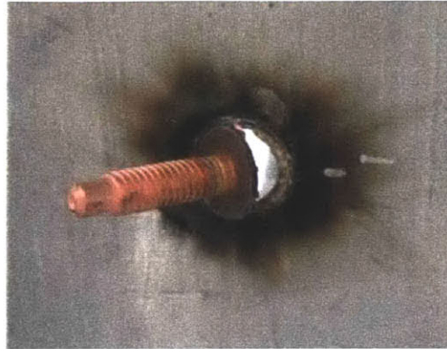
Figure 9. Weld Stud Burn Through
