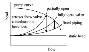
Therefore, at the intermediate valve opening, there is a greater pressure drop across the valve than when fully open. Naturally, this drives a greater flow than would be observed had the pressure drop remained unchanged. The result is an approach of the equal-percentage inherent characteristic toward a linear installed characteristic.
