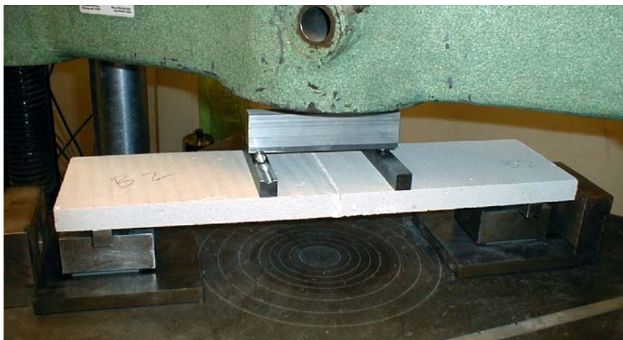
Figure A.19. Photograph of flexural test for bonded AAC/gypsum mortar specimen
