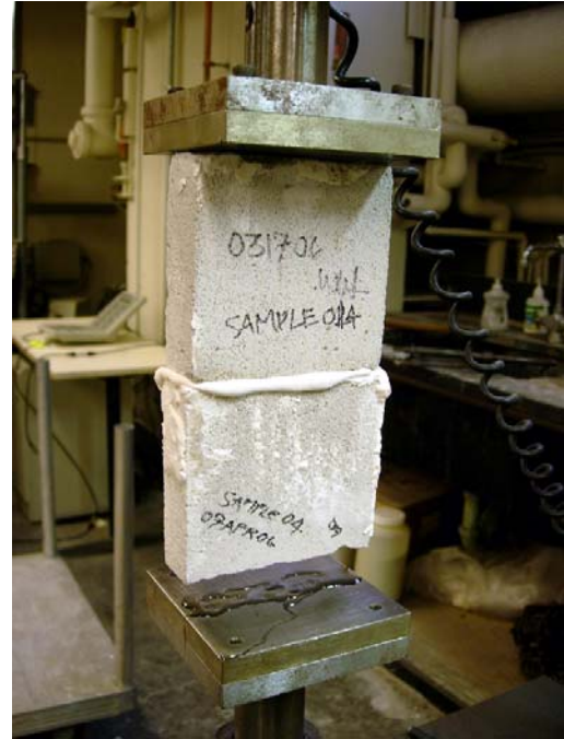
Figure A.20. Left: Direct tension test set-up with two 4 x 4 x 1.25 AAC tiles bonded by a gypsum mortar joint. Right: To minimize unintentional bending forces during testing, the specimens were lowered into an epoxy bed on the lower steel plate in the testing machine.
