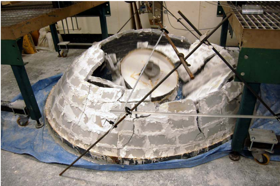
Figure 6.12. Half of Dome 2 collapsed when total displacement of the crown reached almost 1 in.
