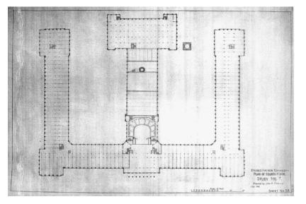
**Fig. 06**: 4<sup>th</sup> floor plan of the academic building. The central series of the structural columns define the double loaded corridor.
