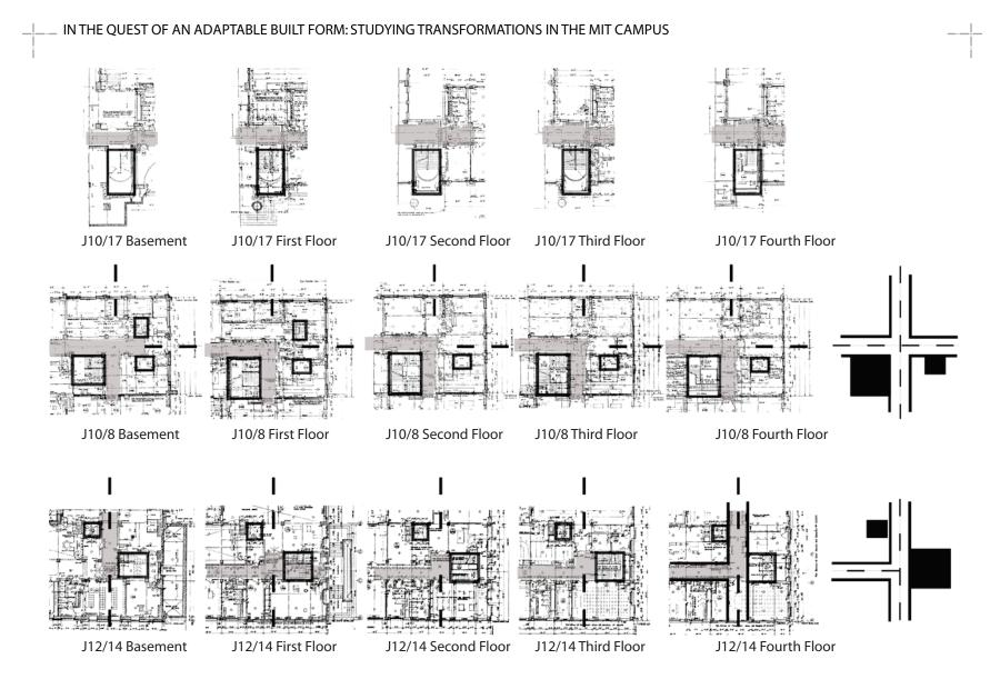
**Fig. 31:** Transparent grey and white outline circulation areas. Black frames show staircases and elevators. Diagrams at the end show possibilities for <u>fut</u>ure expansion.
