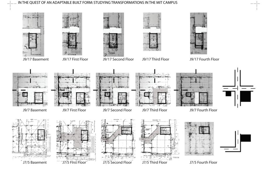
**Fig. 29:** Transparent grey and white outline circulation areas. Black frames show staircases and elevators. Diagrams at the end show possibilities for <u>fut</u>ure expansion.
