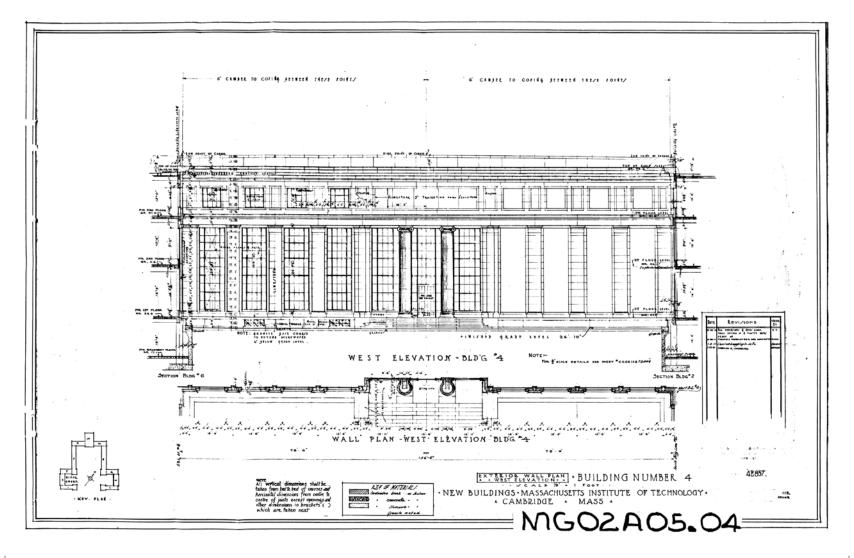
Fig. 39: Facade modeled out with columns and pilasters facing the big Court.
