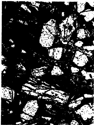
Figure 56a. 50x, as-polished. Unaltered zone.
