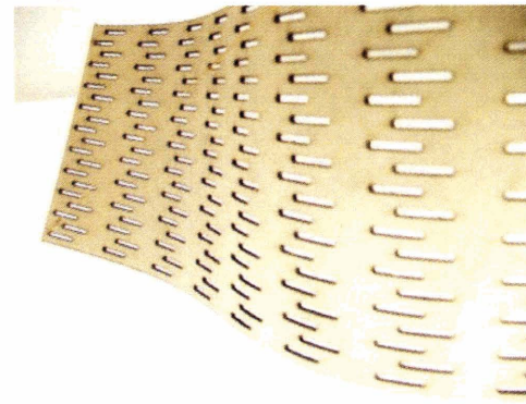
Flexure patterns variations cut on plywood rigid panels and testing elastic properties by applying tensor cables in similar configurations
