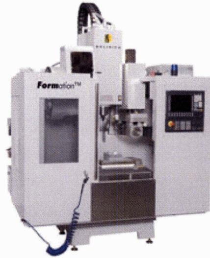
Figure 14 Formation machine which combines both additive and subtractive methods of fabrication
