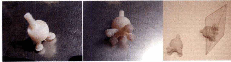
Articulated spider prong joints provide independent operability for each scale feature
