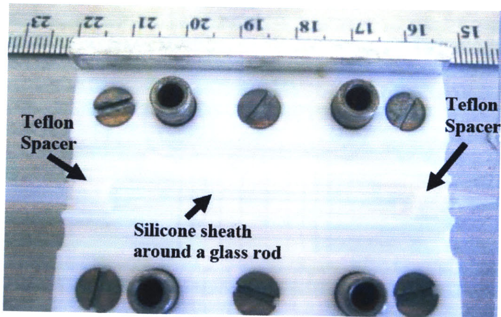
Figure 2.3 – View of the glass rod with a silicone sheath and Teflon spacers in the open mold.
