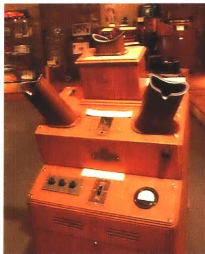
Figure 2.4: Shoe fitting X-ray device. [Image taken from MQMD, 2006]
