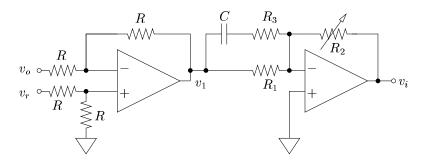
We have constructed the ciruit with  $R_1 = 68 \text{ k}\Omega$  and left off  $R_3$  and C. (You will add them later to make a lead compensator.)
