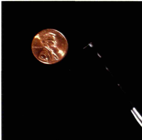
The light sensor: a one-pixel camera.
