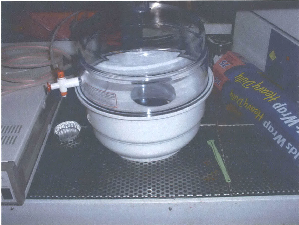
Figure 7-8: Vacuum chamber used for HMDS treatment. A wafer is shown undergoing treatment, which usually lasted for at least half an hour.
