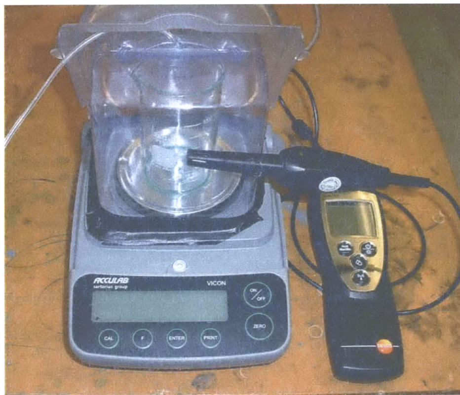
Figure 8-6: Mass Balance Used to Confirm the Accuracy of the Syringe Pump, and Humidity Sensor.
