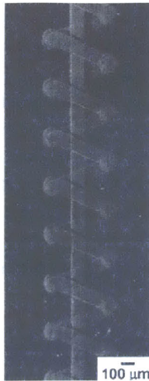
Figure 5-7: Three Dimensional Structures Created via Soft Lithography. From Anderson [2000].
