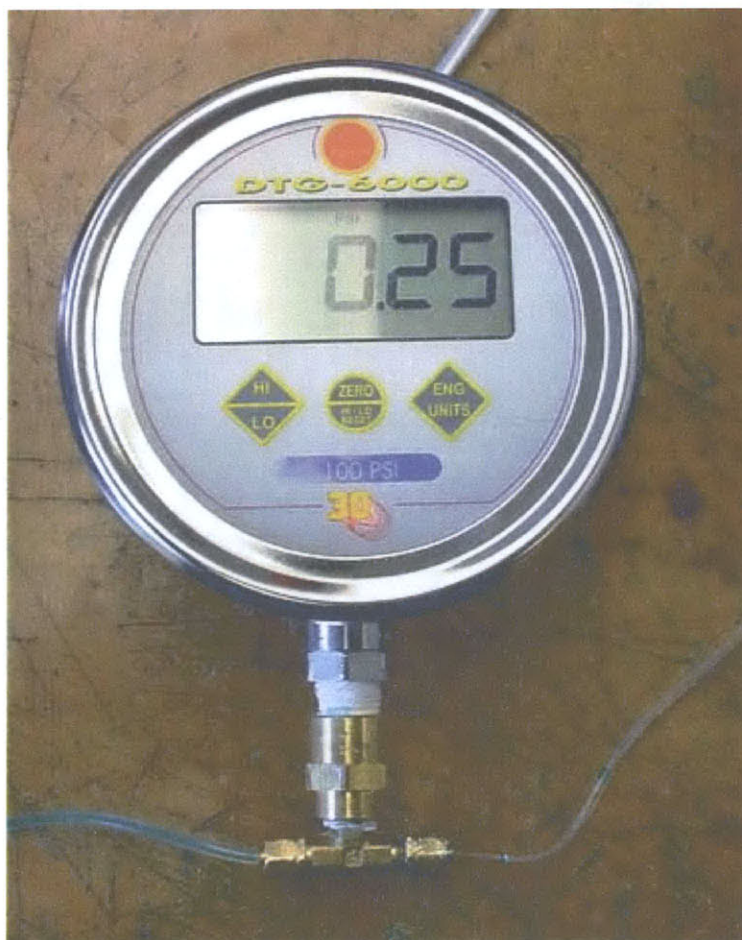
Figure 8-5: Pressure Gauge used to measure pressure drop across the device.
