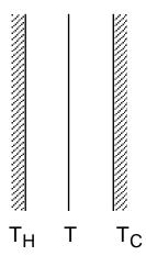
Two parallel plates of infinite extent are separated by a vacuum and maintained at temperatures  $T_H$  and  $T_C$ . The surface of each plate acts as a black body. A thin conducting sheet is suspended in the vacuum as shown in the figure. Heat can be transferred to the sheet only through the vacuum. The sheet has an absorptivity  $\alpha < 1$ , and a power reflectivity  $r = 1 - \alpha$ .
