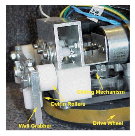
This wall-crawler sliding mechanism moves and allows the wall grabber to tighten on to the side wall. The drive wheel and delrin rollers (connencted to motor) drive the device up the incline. By driving up the side wall, the operator does not have to worry about the horizontal positioning of the device with respect to the scoring slots.
