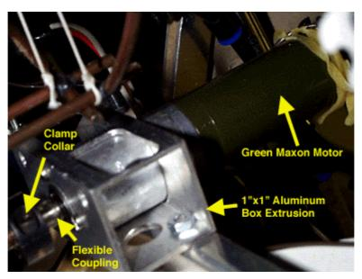
This is good mounting for the green Maxon motor. The box extrusion was drilled to except the mounting holes and the body of the motor. This fixture did take a lot of skill to make. This is a very stiff mounting fixture. Notice the flexible coupling made of the tygon tubing and the clamp collar. Flexible coupling are very important when attaching things to motor shafts.
