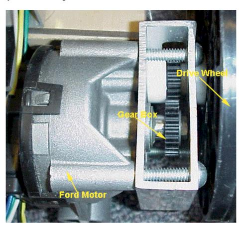
This gear box increases the speed of the Ford Motor (at the expense of torque) which is connected to the drive wheels. When time is a concern, speed is good.
