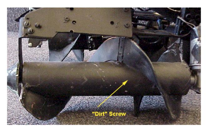
Though this dirt screw was not entirely functional, it was a creative way of propelling the device forward.
