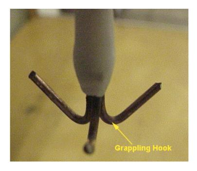
One way of getting a device up an incline without driving up it is to shoot a grappling hook (via a the propulsion of a constant force spring, for example) over the top edge and then wind the device up to it.
