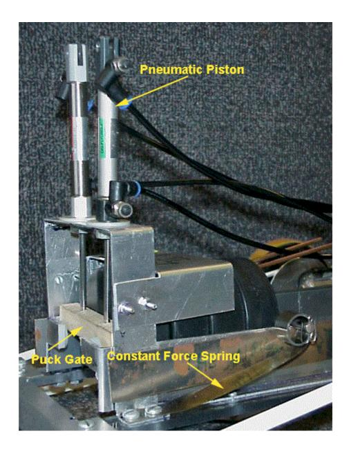
This puck dispensing mechanism is activated via the pneumatic pistons which life the puck gate. When the puck gate is lifted the constant force spring pushes the pucks to the dispensing chute.
