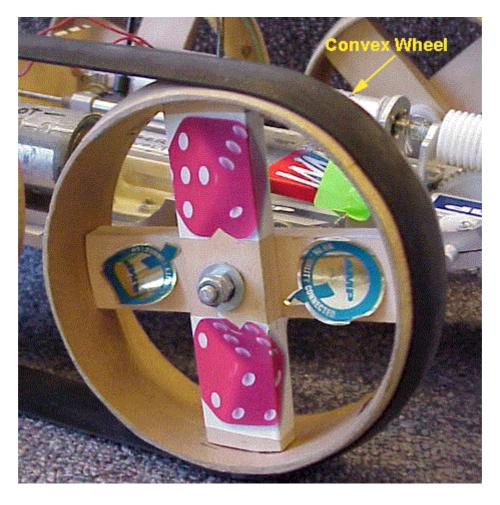
Convex Wheels are GOOD for keeping tracks from slipping.
