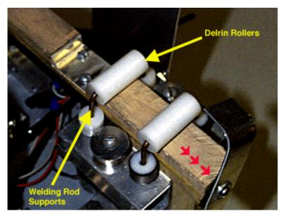
This is a very good sliding mechanism. The delin rollers are much better then just having two flat surfaces slide past each other. This design will support much higher radial load on the sliding part before it binds.
