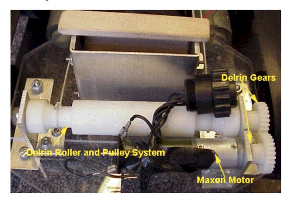
This is a good use of delrin gears. The geared green maxon motor drives the pulley system which pulls the puck gate back, allowing the pucks to exit the storage area.
