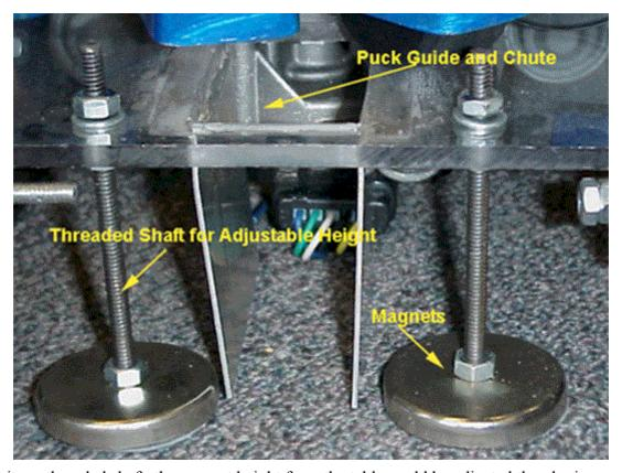
By having a threaded shaft, the magnet height from the table could be adjusted thereby increasing or decreasing the normal force. The puck guides are another good mechanism that prevent jamming of the pucks between the slot in the table and the device.
