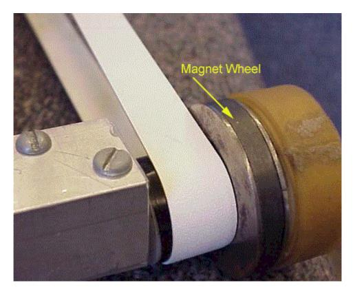
Using magnets as wheels increased the normal force of the device without an overpowering "sticking" effect.
