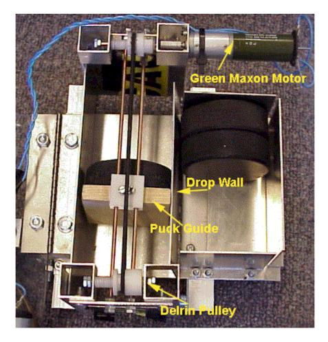
This device has two storage areas of five pucks. The Maxon motor drives the pulley system. As the puck gate reaches the ended of the storage tray, the dividing wall drops down and the other pucks roll into the left bin where the process is repeated.
