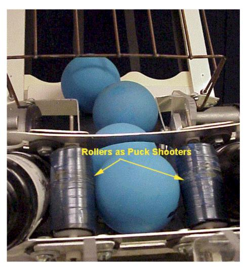
This device has an interesting approach of getting the balls into the scoring area: by shooting them! The delrin rollers mounted on welding rod are powered by a motor and shoot the balls as the fall into
