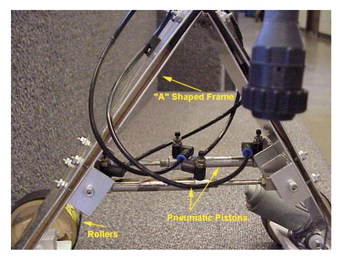
This "A" shaped mechanism is a creative simulation of "walking". With the assistance of the rollers, the pistons push the frame out further. When the pistons are deactivated, the back end of the frame is edges its way back to the starting angle.... and the process starts over.
