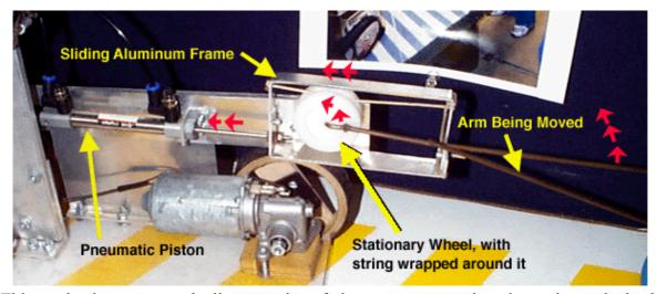
This mechanism converts the linear motion of piston to rotary motion via a string and wheel.
