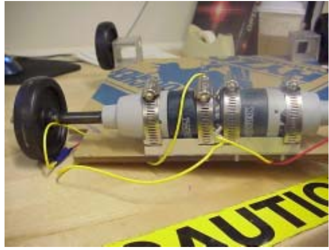
A clever way to mount the Black & Decker motors using the 1.5" Al. box extrusion and hose clamps. The only manufacturing required was 3 band saw cuts per mount. Simple and functional, the perfect combination.
