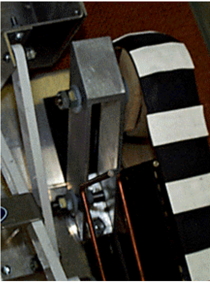
The 1" x 3" aluminum box beam cut in to parallelogram.
