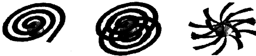
Figure 2. Spiral energy harvesters designed by Professor Kim's group at MIT 5 .
