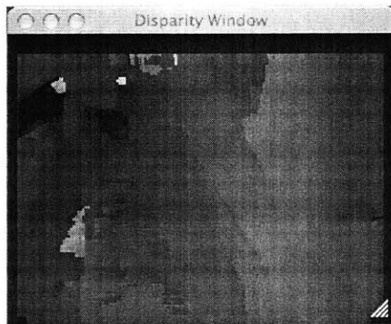
Figure 5-2: Depth map computed with image pyramid
