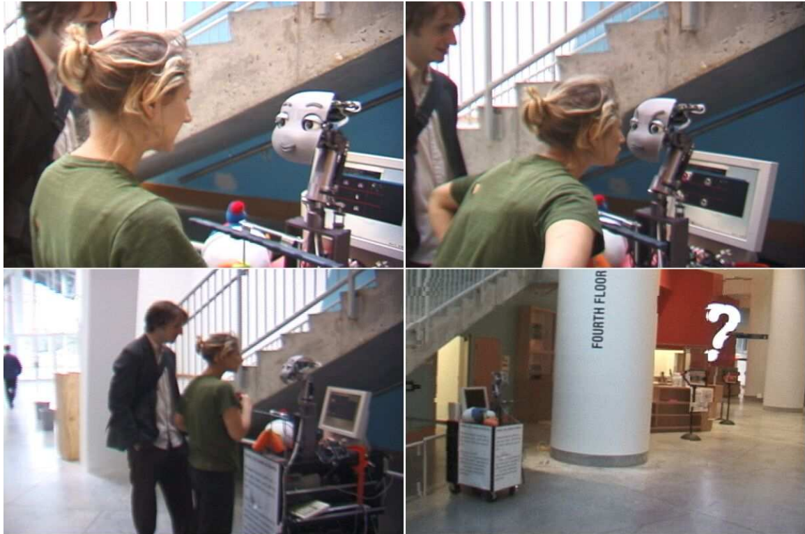
Figure 3-12: A sample interaction session on day 5 of the experiment. The robot ran continuously for 7 hours in a different public location each day. A written sign was placed on the robot: “ Hello, my name is Mertz. Please interact with me. I can see, hear, and will try to mimic what you say to me.” Some bright colored toys are available around the robot. On the bottom right corner is a full-view of the robot’s platform in the lobby of the MIT Stata Center.
