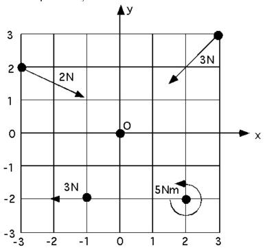
Consider the system of forces and couples acting in the directions indicated on the  $6m \times 6m$  grid shown above. Calculate:
