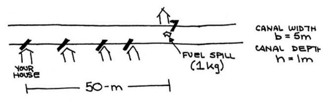
YOU OWN A HOUSE AND DOCK ALONG A LONG BOAT CANAL. ONE DAN YOUR NEIGHBOR HAS A SMALL FUEL SPILL. DUE TO THE BOAT TRAFFIC, THE DIFFUSIVITY IN THE CANAL IS QUITE HIGH ,D=0.01 THE CURRENT IN THE CANAL IS NEGLIGIBLE, SUCH THAT THE FUEL IS TRANSPORTED TO YOUR HOUSE BY DIFFUS ONLY. ASSUME THE FUEL MIXES RAPID ACROSS THE WIDTH AND DEPTH.
