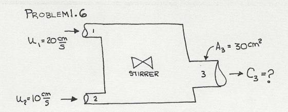
TWO PIPES, EACH OF 10 cm² cross-section, CARY WATER INTO A MIXING CHAMBER. THE UPPER PIPE CARRIES WATER SATURATED IN OXYGEN (C1 = 9 mg/e), AND THE LOWER PIPE CARRIES DEOXYGENATED WATER (C2 = 0 mg/e). A STIRRER WITHIN THE CHAMBER RAPIDLY MIXES THE TWO STREAMS, SUCH THAT THE CONCENTRATION IN THE TANK IS SPATIALLY UNI FORM. ASSUMING THE SYSTEM IS AT STEADY STATE, WHAT IS C3?
