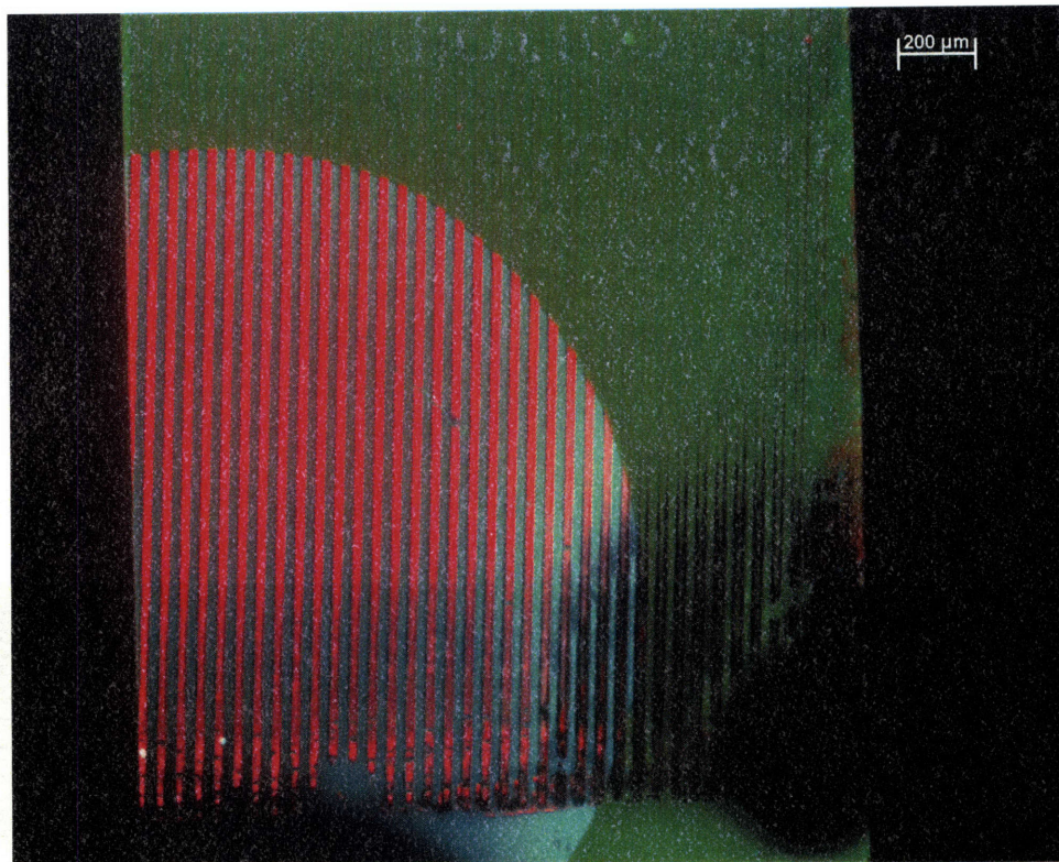
Figure 6-16: Lines of red quantum dots printed atop a full-plane green quantum dot film. An area where the PDMS did not contact the substrate when printing the green QDs shows the red QD emission as well as the organic. However, in all other areas, the luminescence of the red dots is much reduced.
