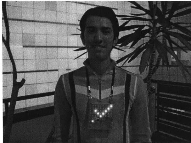
Figure 1. The UbER-Badge records accelerometer and audio signals as well as IR encounters with other badges and fixed beacons called Squirts.
