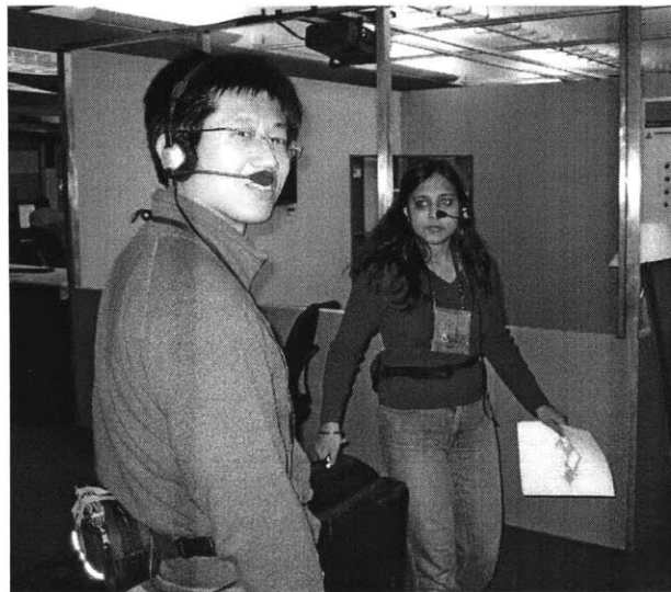
Figure 2. Subjects are wearing a hybrid UbER-Badge / Sharp Zaurus PDA system that includes accelerometers on waist and chest, a close-talking microphone, an IR transceiver, and a Bluetooth scanner.
