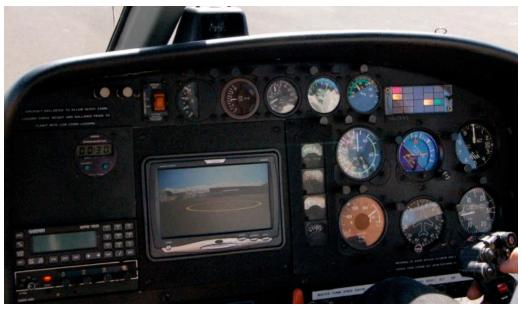
Figure 7: Air tour helicopter panel with video monitor
