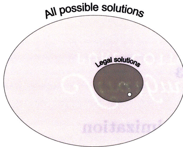
Figure 3-1: An abstract depiction of a heuristic’s task. The large, light gray circle represents the space of all possible solutions to a compiler problem. The heuristic first finds a subset of solutions, represented by the dark gray circle, that will generate legal code. The heuristic’s policy then chooses a single solution, denoted by the small white circle, from this subset.
