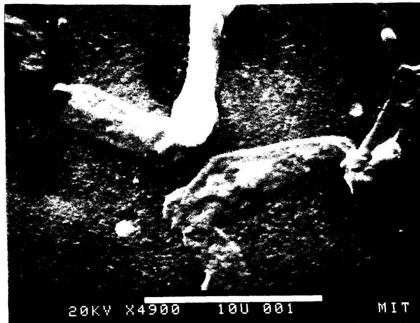
Fig. 6. Collapsed mycelium-like cell wall. Picture taken by scanning electron microscope(x4900).
