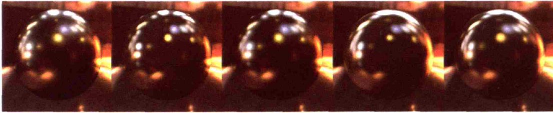
Figure 3-5: Fitting the measured BRDF "nickel" with the multi-lobe Cook-Torrance and Lafortune models. Left to Right: Input, Cook-Torrance 1 lobe, Cook-Torrance 2 lobes, Lafortune 1 lobe, Lafortune 2 lobes.
