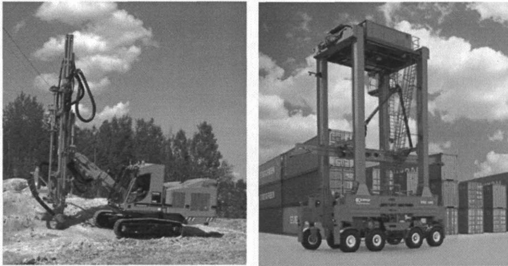
Figure 4-4 Among Tampere's leading machinery companies are those specialized in mobile machinery for various industries. Shown to the left, one of Sandvik-Tamrock's rock-drilling machines. To the right, a container handler machine made by Kalmar Cargotec. Sources: Sandvik MediaBase and Cargotec ImageBank.
