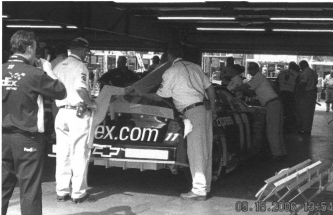
Figure 5-7 NASCAR officials using one of the 33 templates (as of 9/15/06) to make sure that each racecar's body meets the specifications set by the rules. Author's photograph. Loudon International Speedway, NH. 9/15/06.
