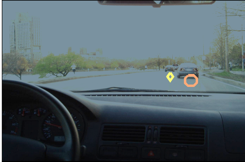
Figure 2-16: An example implementation of multi-stage directional alerting (1 of 3); locational stimulus highlights objects in the environment (diamond and octagon on windshield).
