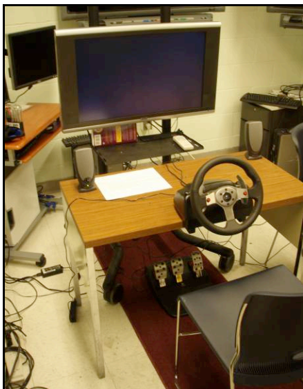
Figure 3-8: The driving simulator.
