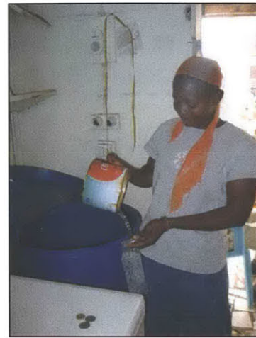
Figure 2.6: Hand-tied sachet water being manually filled
