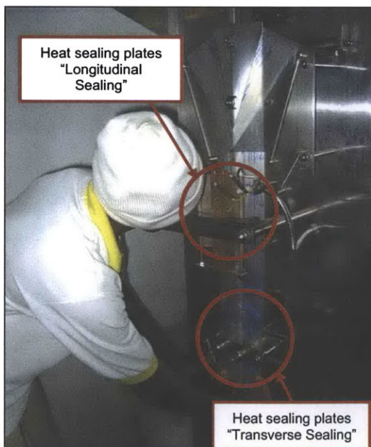
Figure 6.12: 0.5m of sachet rolls sealed longitudinally and at one end
