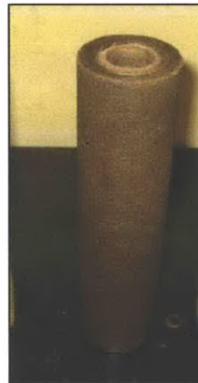
Figure 6.8: Fiber filter cartridge (used)
