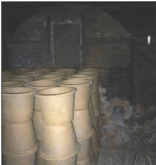
Figure 1.7: Filter awaiting firing in kiln
