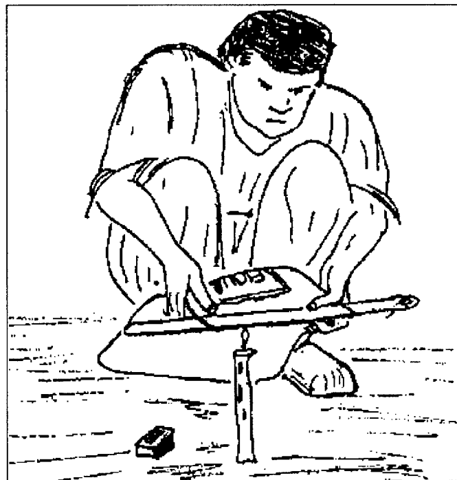
Figure 7.15: Candle and hacksaw blade method of sealing plastic bags (FAO, 1994)
