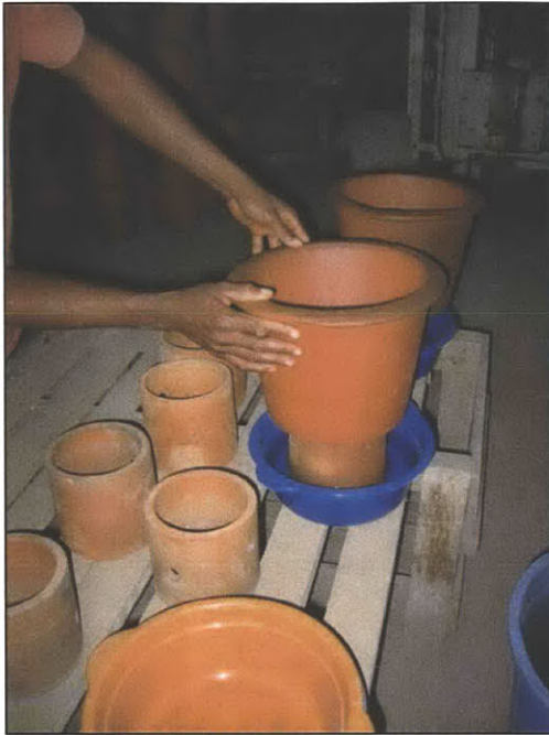
Figure 1.9: Testing filter flow
