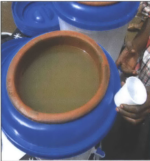
Figure 1.11: Filter in use. Filtrate comparison with raw water
