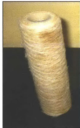
Figure 6.7: Yarn filter cartridge (used)
