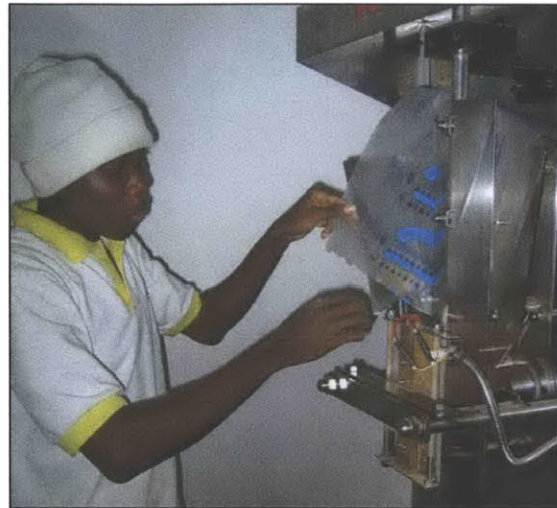
Figure 6.11: Polythene rolls adjusted by folding on base board of bag former
