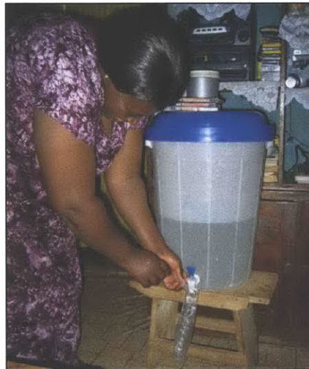
Figure 7.10: Ceramic pot filter use in hand-tied sachet-water production
