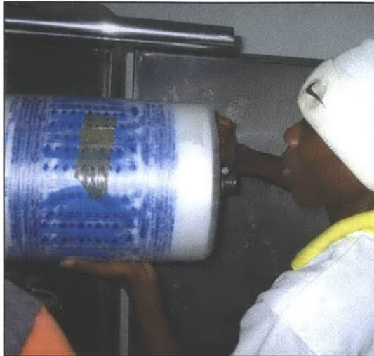
Figure 6.10: Loading of polythene rolls in sachet machine
