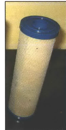
Figure 6.9: Matrix carbon filter cartridge (used)
