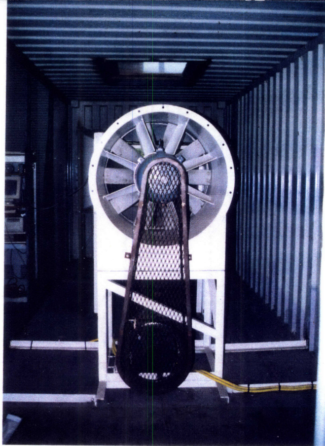
Figure 5-1. Photographs of the windtunnel
