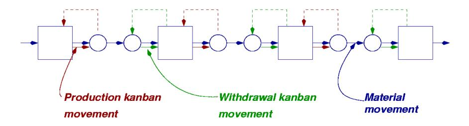
When a buffer has a free withdrawal kanban, a part moves to it from the upstream buffer, and a production kanban moves to the machine.
