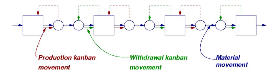
After the operation, the withdrawal kanban returns to the upstream buffer, and a part and a production kanban move to the downstream buffer.
