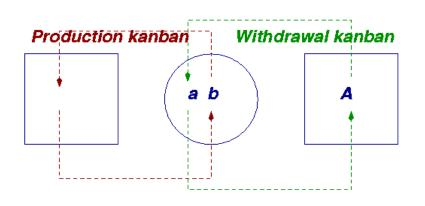
Unattached production kanbans are the signal to tell upstream stage how much to produce.
