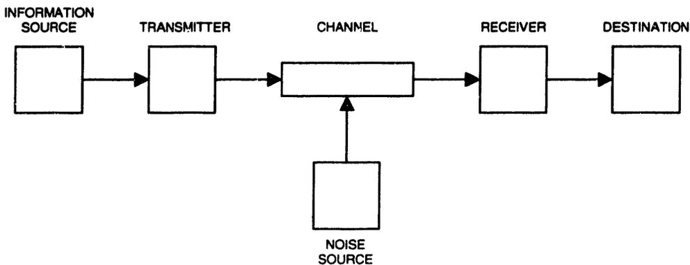
**COMMUNICATION BLOCKS** Shannon's classic schematic diagram of a general communication system. All practical systems can be broken down into parts that perform the same functions as these boxes.
