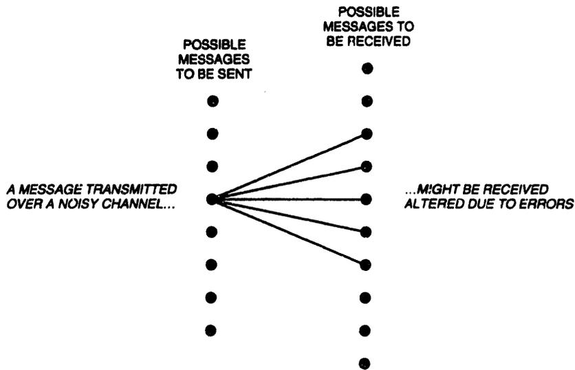
**FAN DIAGRAM** The figure shows a typical “fan diagram,” as this kind of schematic drawing was known to MIT graduate students in the 1950s. The points on the left represent the messages to be sent. Due to errors in the channel, a transmitted message can arrive altered (points on the right connected by lines).
