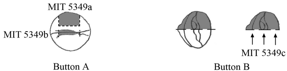
Figure 5.4.6.v: Samples removed from buttons. Samples MIT 5349a and MIT 5349b were removed from Button A for bulk composition analysis. Sample MIT 5349c was removed for metallographic analysis and was mounted transversely as noted.
