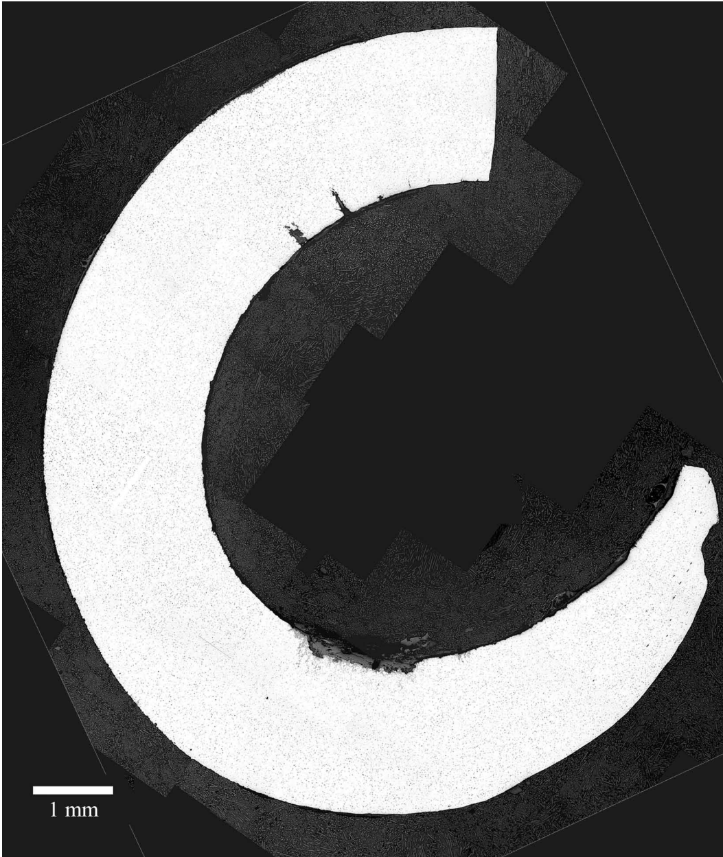
Figure 5.2.3.ix: Navicular fibula (MIT 5348/Peabody 40-77-40/13285). Longitudinal cross section, as polished. The longitudinal cross section shows that the metal has been coiled into an oval-shaped spring. Microstructural features of interest include small porosities homogenously distributed throughout the sample, elongated gray copper sulfide inclusions oriented parallel to the longitudinal axis, and a few surface cracks perpendicular to the longitudinal axis. These cracks most likely stem from repeated flexing of the spring (MIT Images 5348b-01-29).
