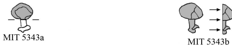
Figure 5.3.1.iv: Rivets (MIT 5343). Samples removed from rivets. MIT 5343a was removed from Rivet A for bulk compositional analysis. Rivet B was taken in its entirety as MIT 5343b for metallographic analysis. It was mounted longitudinally and ground down until the entire center plane of the rivet was exposed.
