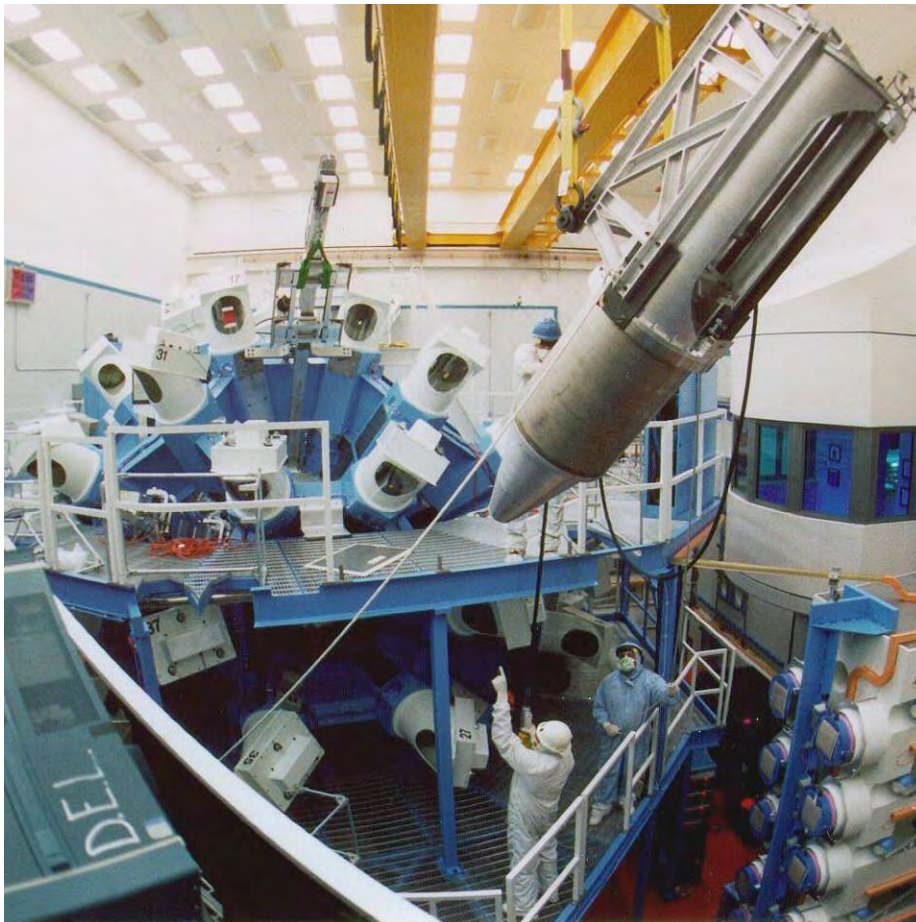
Figure 2-12: The OMEGA target bay during the installation of the CPS-2 diagnostic. The CPS-2 housing contains 4000 lbs of lead and polyethylene shielding to reduce the neutron background on the detectors.
