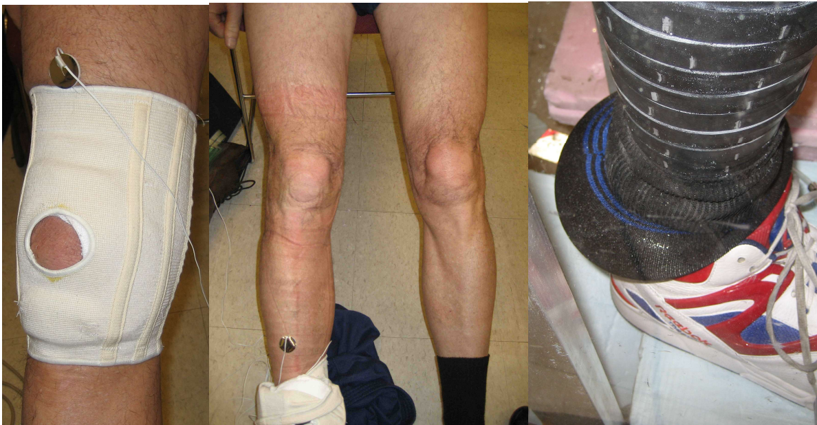
Figure 67: (left) Leg of Subject 2 in the knee brace Figure 68: (center) Legs of Subject 2 after the test with the knee brace Figure 69: (right) Sock of Subject 2 swelling outside the restraining layer
