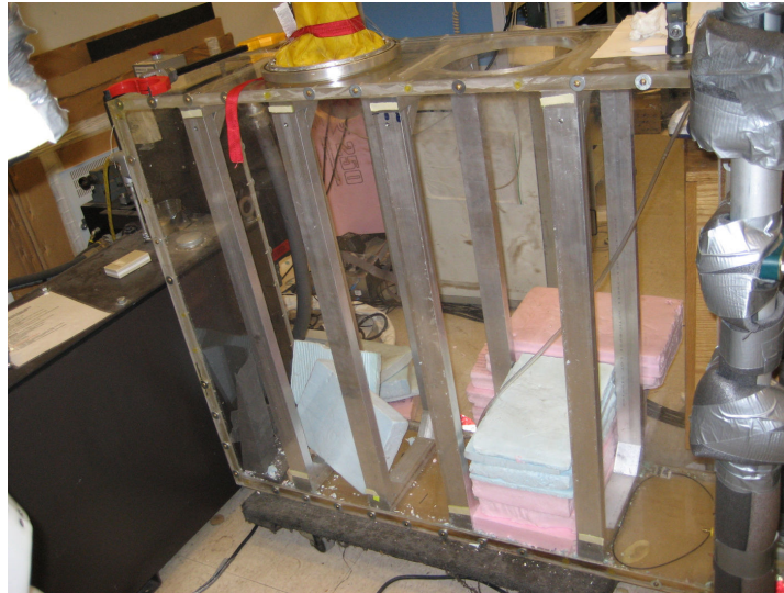
Figure 46: Low pressure chamber
