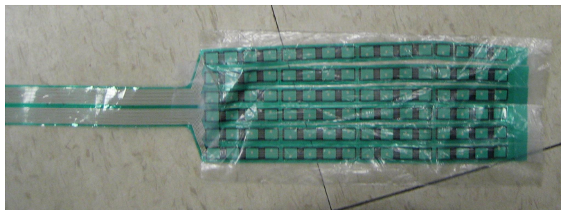
Figure 32: TekScan Model 9801 sensor
