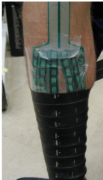
Figure 41: TekScan sensor wrinkling from the pull of the bands
