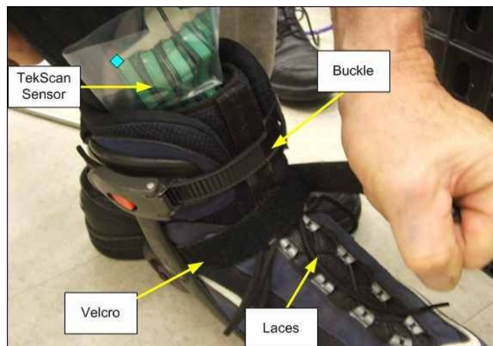
Figure 10: Roller blade testing
