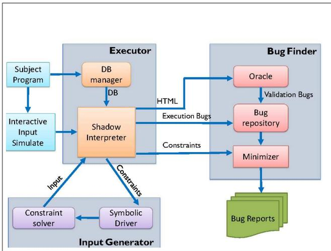
Figure 4: Illustration of the architecture of Apollo.
