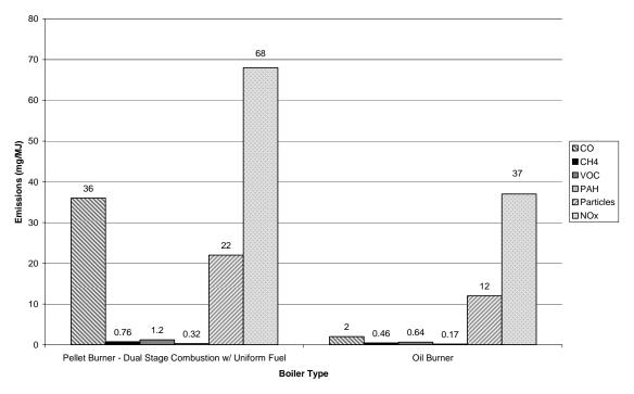
Air Emissions Comparison for Pellet and Oil Burner
