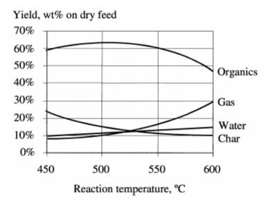
Typical yields of organic liquid, reaction water, gas and char from fast pyrolysis of wood, wt% on dry feed basis. Figure 11: Fast Pyrolysis Yield as a Function of Reactor Temperature [Bridgwater, 1999, p1480]
