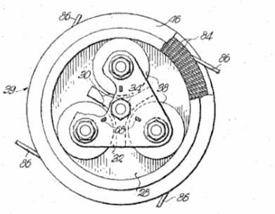
Figure 10: Image of a Rotary Pellet Press [Wenger, 1967]
