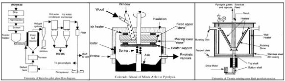
Figure 12: Pyrolysis Reactor Types: Fluidized Bed, Ablative, and Cyclone (from left to right) [Bridgwater, 2000, pp 57, 23, 54]
