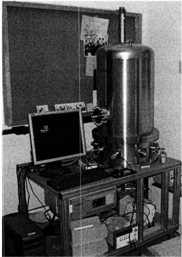
Figure 65. The high-temperature vacuum thermoelectric test bench (a.k.a. Shrek).
