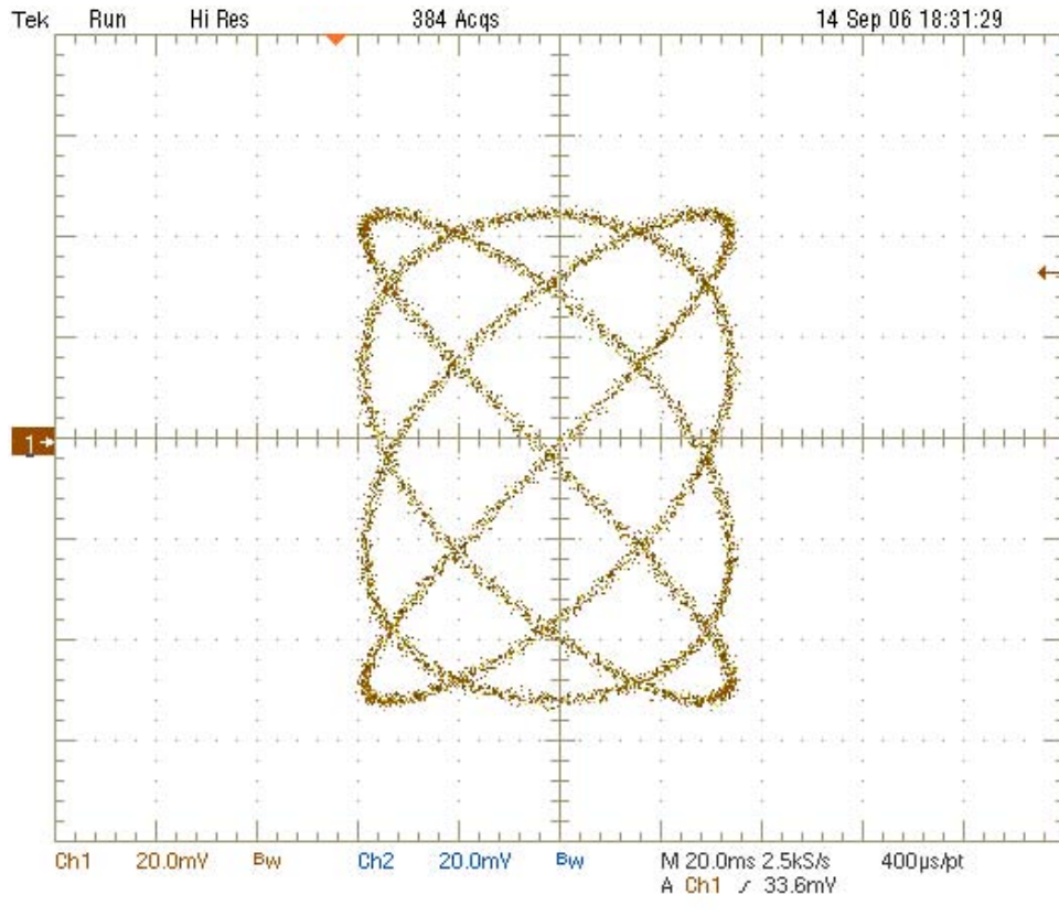
Figure 5-39: Lincoln Laboratory logo lissajous figure drawn at 500 Hz under dual-axis operation.
