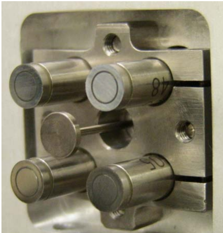
Figure 4-8: Probe clamp with probes and axial flexure installed.
