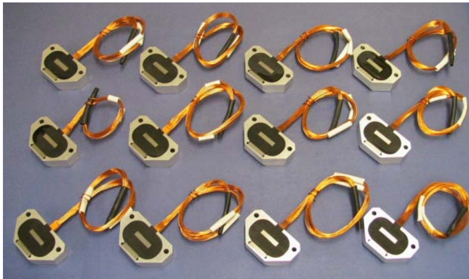
Figure 4-13: Finished actuator halves after final grind.
