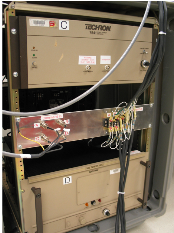
Figure 4-22: Model 7541 (top) and 7560 (bottom) power amplifiers mounted in their racks during AFSM testing. Note also the shield terminations on the four cables at the output terminal block at middle-right.
