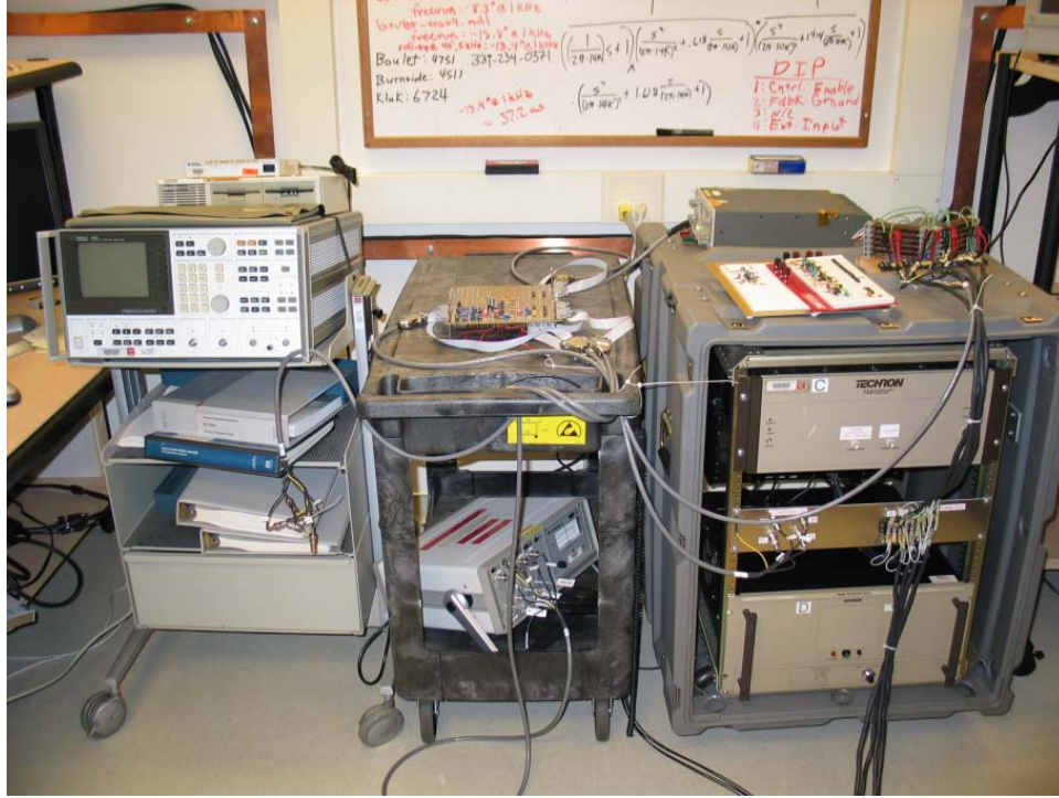
Figure 5-1: The AFSM electronic support and test hardware at Lincoln Laboratory. The HP 3562A DSA is on the left.
