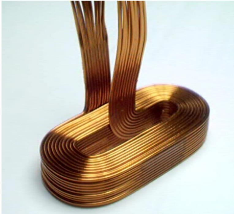
Figure 4-10: A finished coil assembly after forming and bonding. Photo courtesy of Fred Sommerhalter.
