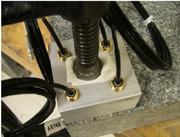
Figure 4-7: The capacitance probes installed in the alignment fixture during bonding of the probe housings (threaded brass parts over the probes).
