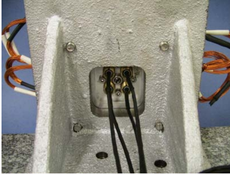
Figure 4-21: Rear view of the AFSM assembly showing the installed capacitance probes.
