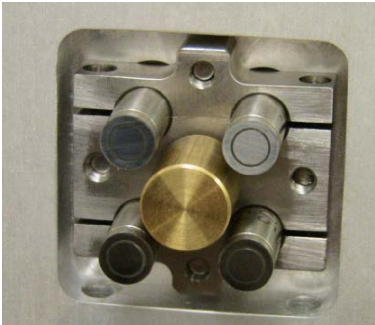
Figure 4-15: The probe sensor clamp installed in the base plate using an alignment pin (brass part in the center). Note the access holes in the base plate for the clamp screws at the bottom of the figure.
