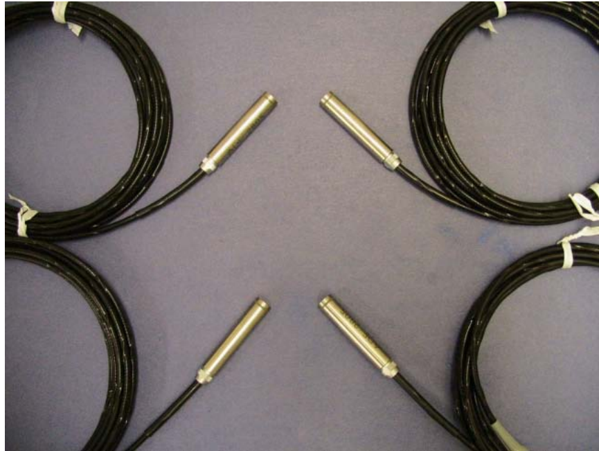
Figure 4-28: The set of four capacitance probes prior to installation in the AFSM.
