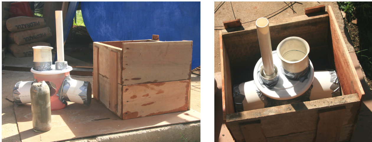
Figure 5: Wooden mold and sacrificial mold core that holds the shape of the cavity for the tensioner and bearing that sits at the bottom of the well.
