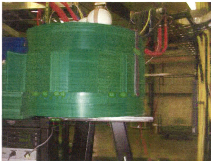
Figure 6.14: Borated polyethylene gas target shielding
