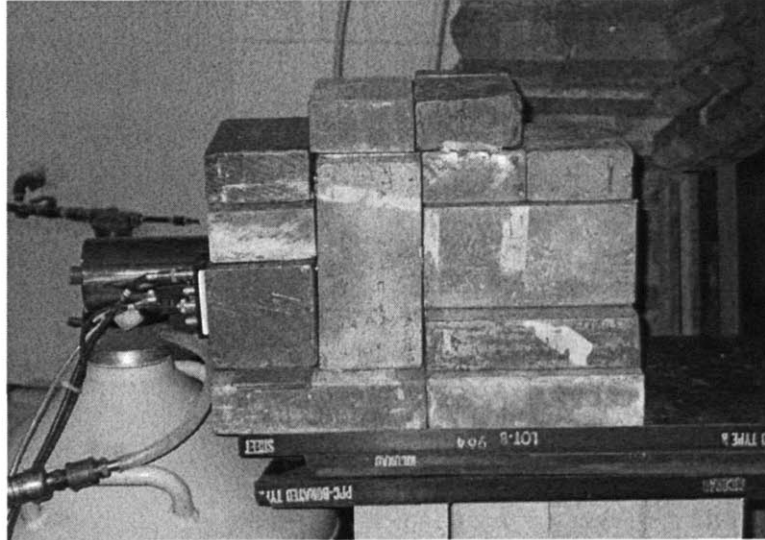
Figure 4.6: Gamma ray detector and shielding arrangement
