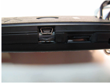
Figure 4-8: Badge’s side view: miniUSB port, tri-directional switch, and microSD card socket.
