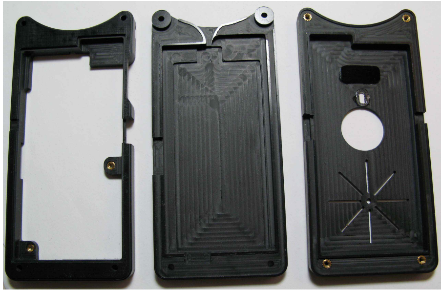
Figure 4-7: Middle, back and front layers of the badge enclosure.
