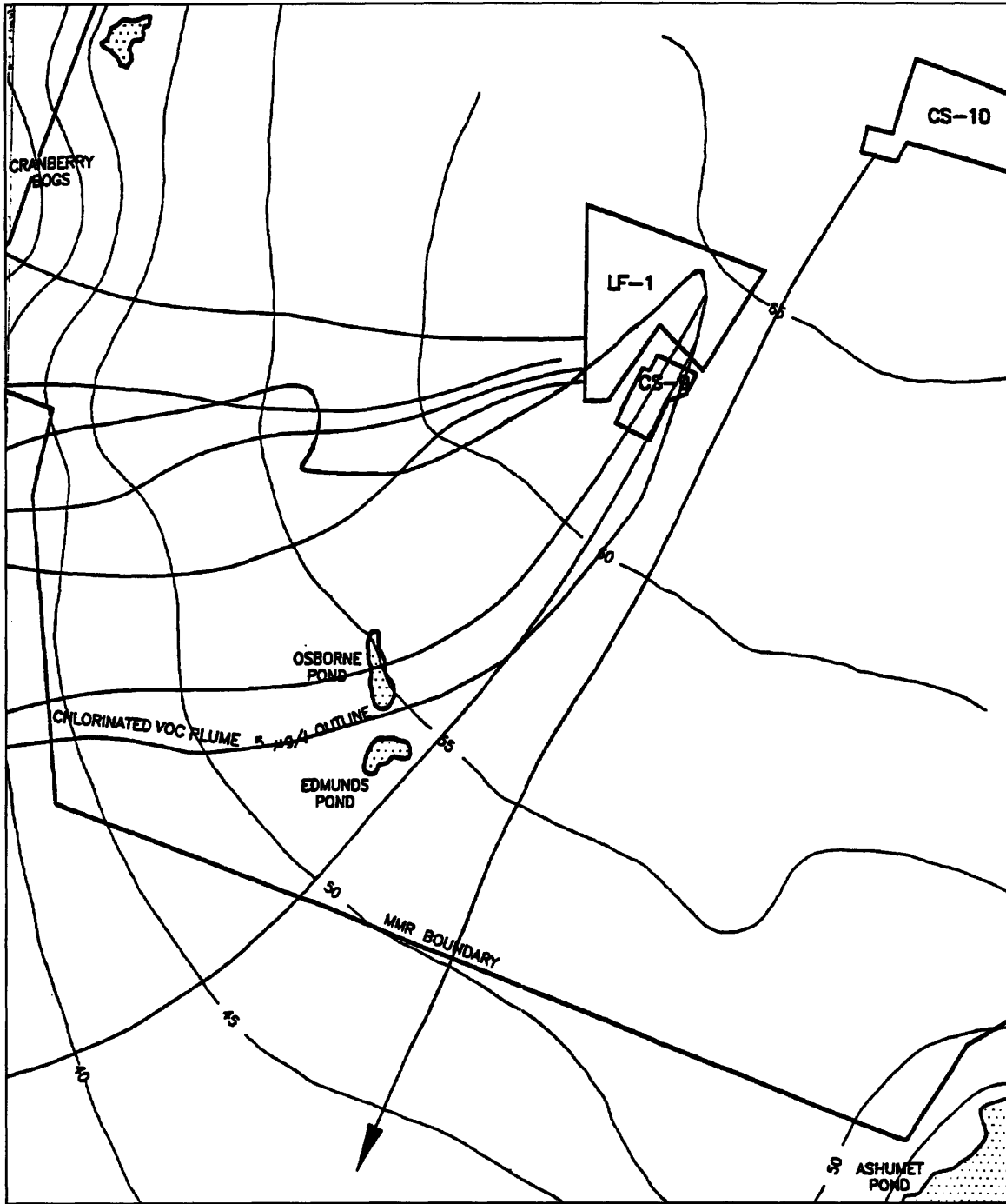
Figure 3-5 Water Table Elevations and Flowlines in the LF-1 Area (Stone & Webster, 1996a)
