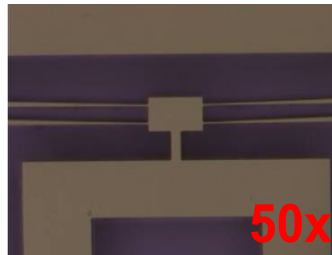
B: GRIN lens shuttle amplification flexure
