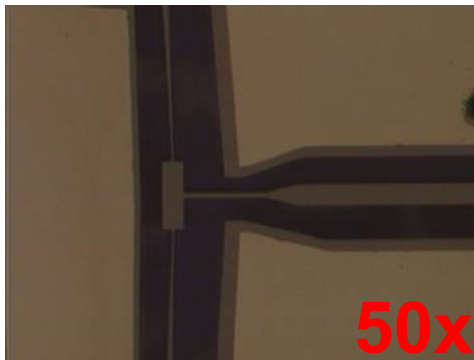
A: Prism shuttle amplification flexure
