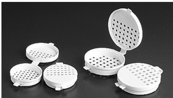
Figure 2.2 Polypropylene histology cassette used to support agarose membranes during the activation and attachment processes. (Histo-prep Tissue Capsules, #15-182-219; Fisher, Hampton, NH)
