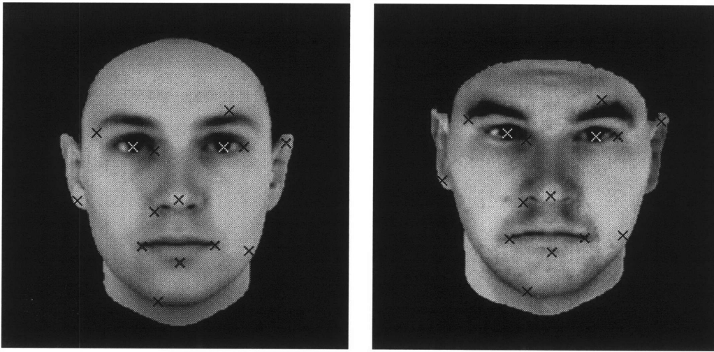
Figure 8.4: The left image shows the reference face with a number of points marked with an “X”. The right image shows the corresponding points on a prototype face. These correspondences were found using the automatic bootstrapping algorithm.
