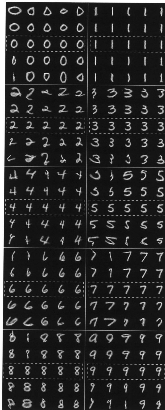
Figure 8.5: For each of the 10 digits the figure shows the first five shape eigenvectors (left to right) of the model (obtained from 250 prototypical digits). Each column displays how each shape eigenvector changes relative to the average digit (in dashed box). The range of the coefficient ranges from +5 (top) to -5 standard deviations (bottom) of each eigenvector.
