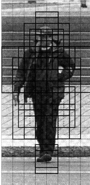
Figure 3-5: The significant wavelet bases for pedestrian detection that are uncovered through our learning strategy, overlaid on an example image of a pedestrian.
