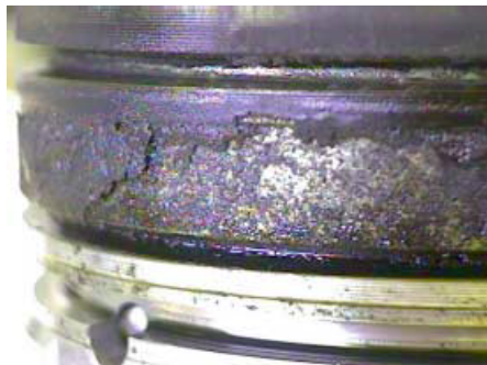
Figure 2: Piston with a substantial carbon deposit problem.
